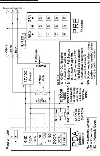
NOTE: The 3 1N4004 diodes referred to in the wiring diagram are packaged with the PRDA.
